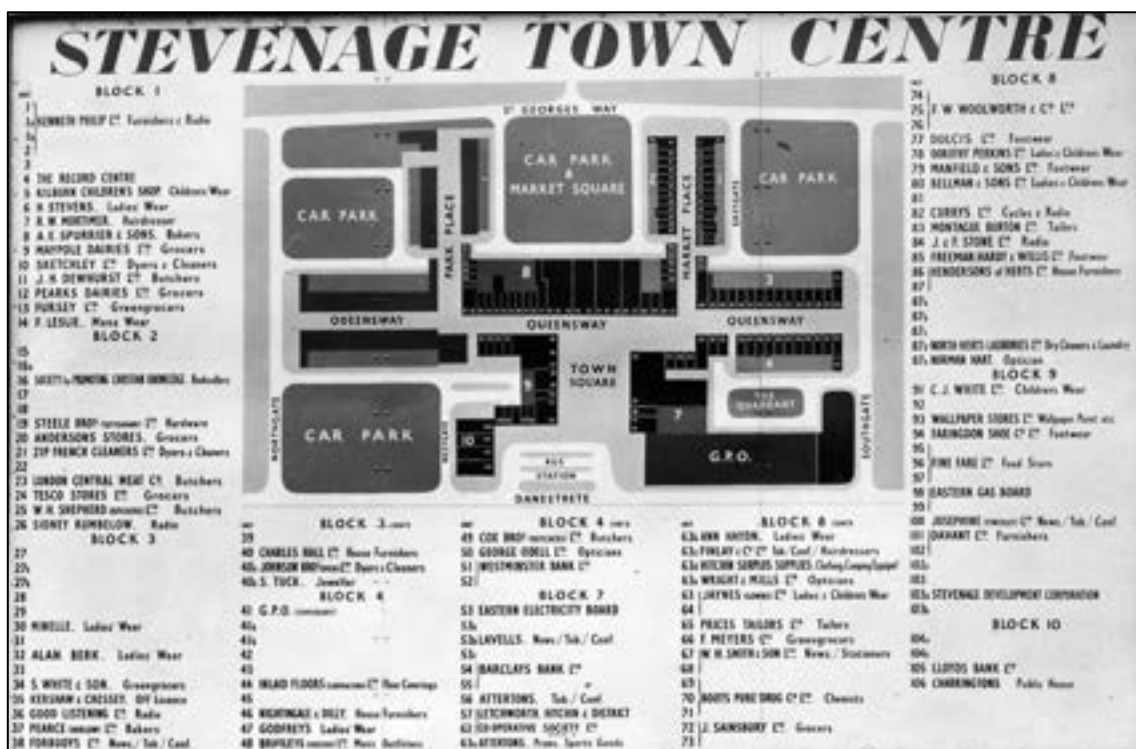
Figure 4: Plan of Stevenage Town Centre in 1958. Despite the major pedestrianised avenues and Town Square, large surface-level carparks resulting from the designer’s modernist tendencies disrupt the urban fabric and complicate contemporary redevelopment (Mortimer, 1958).
